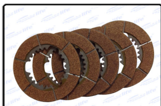
Part No : ATL AP O-24 Description : CLUTCH PLATE SET CORK Suitable For : APE MRP : 90
